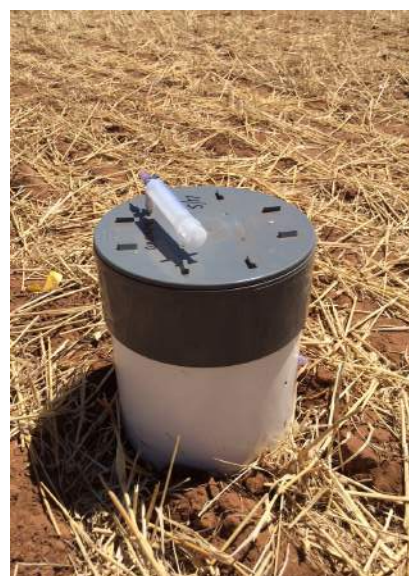
Chamber to collect samples of air that are analysed for nitrous oxide. Photo taken at WANTFA's Cunderdin long-term site.
